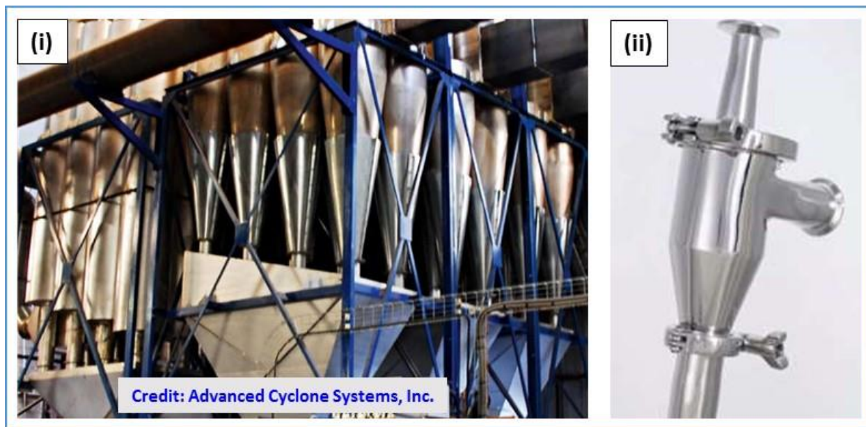
Figure 23. Application spectrum of cyclone technology for nano-particulate collection by ACS, Inc.: (i) emission control—large, multiple units designed for high volume and/or high temperatures [ref. 46]; and (ii) product recovery—smaller, individual units designed for efficiency and cleanliness [ref. 47].
