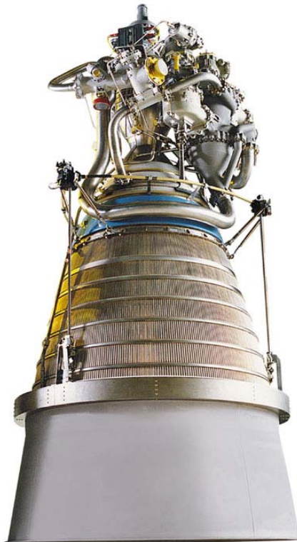
Figure 12-33. RL-10 Engine with extendable carbon-carbon nozzle extension (NASA photo archives)
