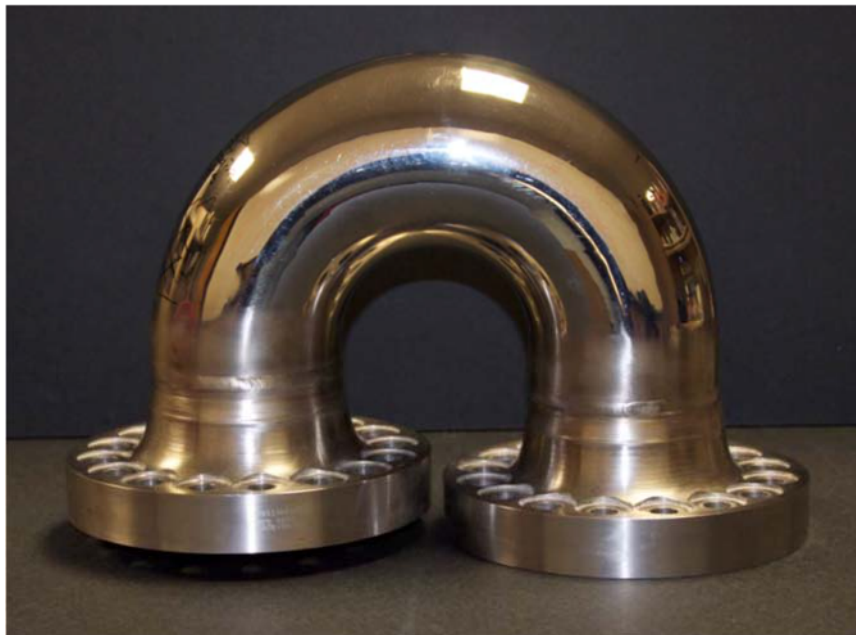
Figure 12-50 J-2X DMLS Gas Generator Discharge Duct (NASA/MSFC photo)
