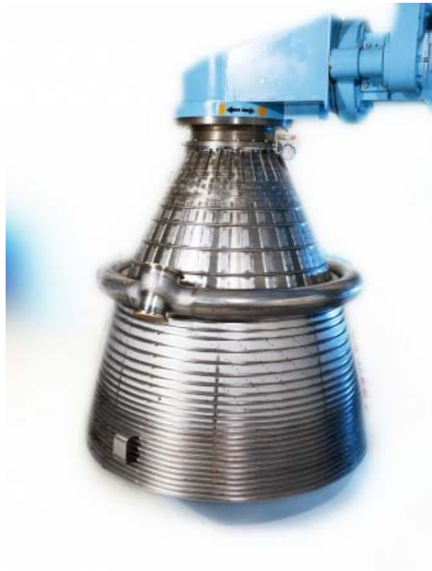
Figure 12-27. Completed Volvo Aero Tubular nozzle. (Courtesy of Volvo Aero)
