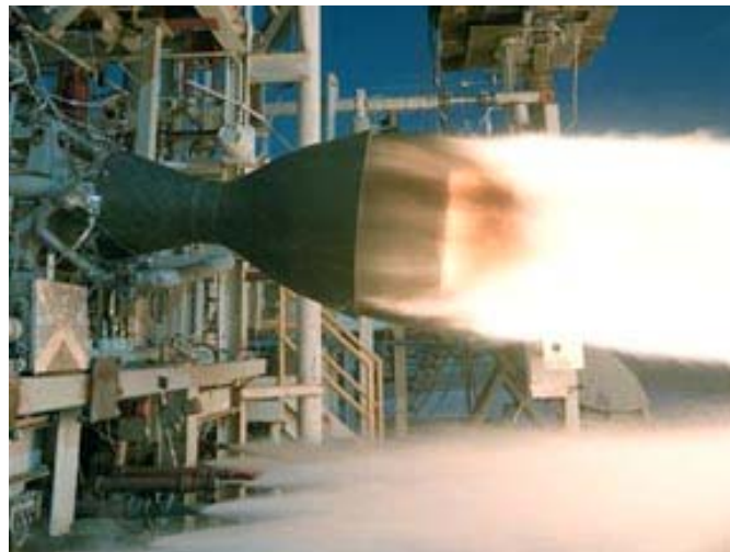
Figure 12-35. Fastrac Engine Hot-Fre Test at NASA/ Marshall Center (Source: NASA/MSFC)
