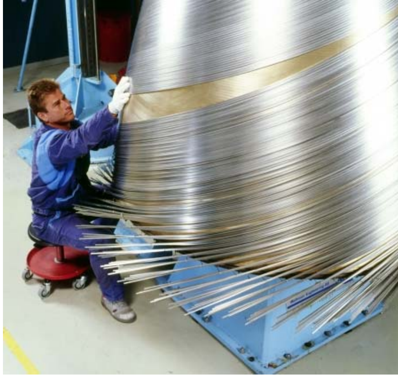
Figure 12.26. Assembly of a Volvo Aero tubular nozzle. (Courtesy of Volvo Aero)
