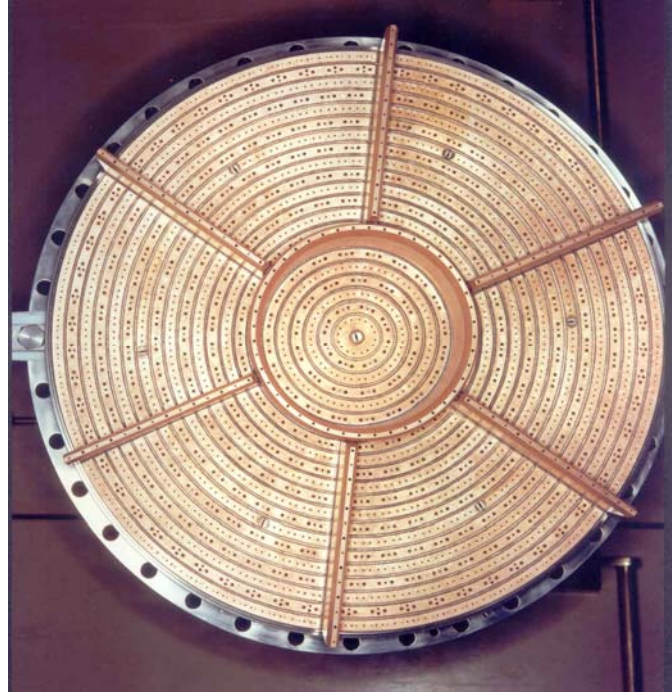
Figure 12-12. A baffled, concentric-ring injector for an Atlas launch vehicle. OFHC Copper rings brazed into a stainless steel body. (NASA archives)
