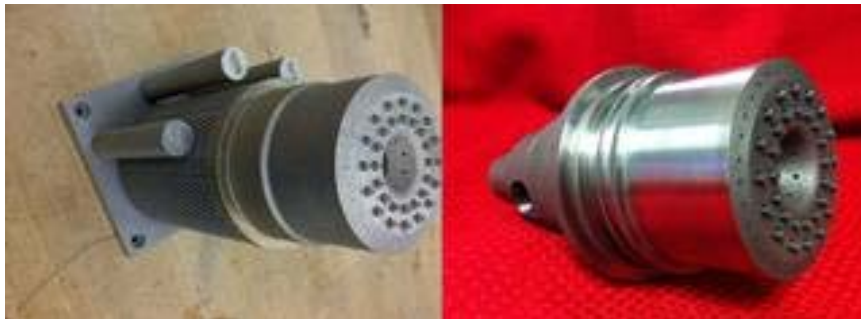
Figure 12-15 Left: 3-D printed rocket injector as it looked immediately after it was removed from the selected laser melting printer. Right: Injector after inspection and polishing. (Source: NASA/MSFC)
