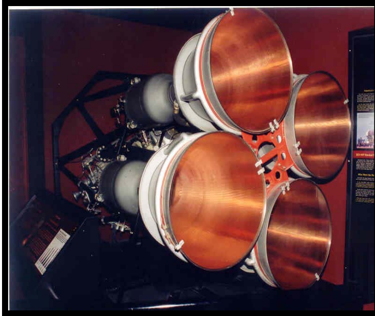
Figure 12-22. Photo of a Russian RD107 Engine clearly showing the copper alloy inner liner of the nozzles. (Photo taken at the Kansas Cosmosphere museum)
