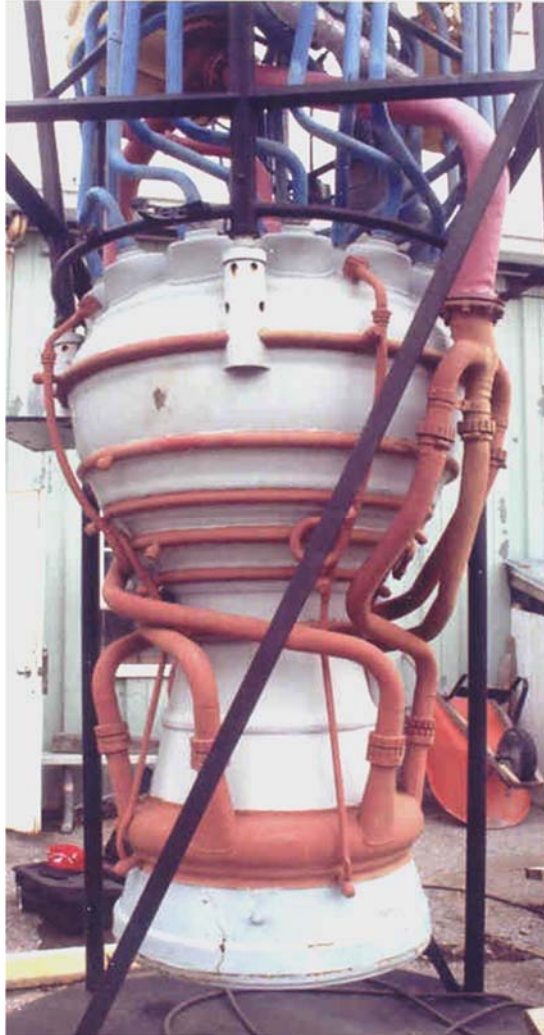
Figure 12-18: V-2 Combustion Chamber and Nozzle. Red colored tubes are fuel lines made of steel. Blue colored tubes at top of photo are liquid oxygen lines made of aluminum alloy. (Photo taken at the Huntsville Space Museum restoration shop)
