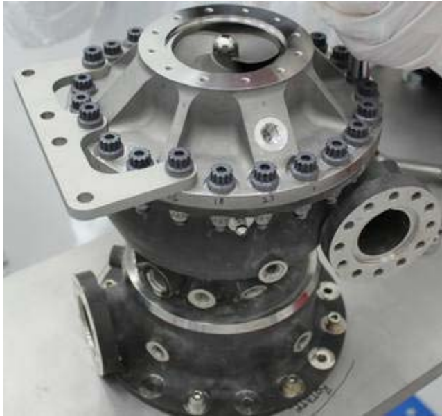
Figure 12-45. 3-D Printed Liquid Hydrogen Turbopump (Source NASA/MSFC)
