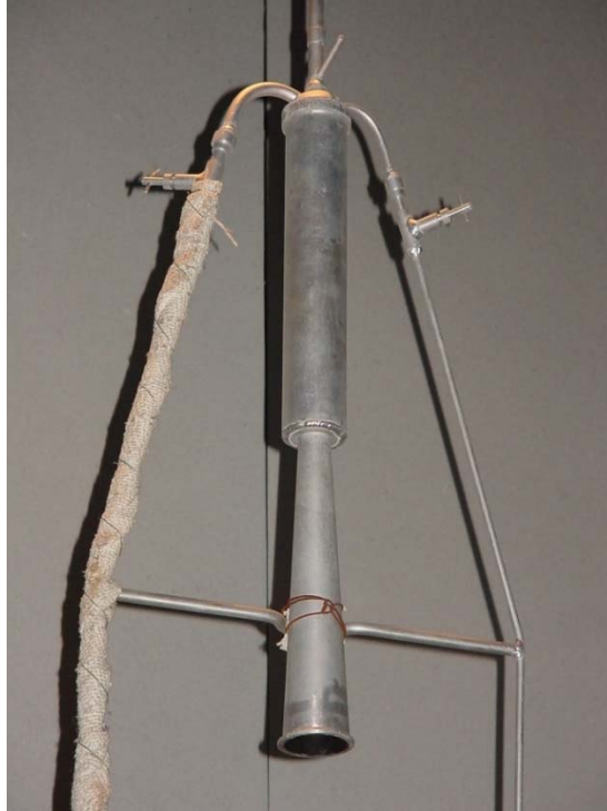
Figure 12-16: A replica of Dr. Robert H. Goddard's first combustion chamber and nozzle. Combustion chamber was aluminum with a layered liner of asbestos and alumina. The nozzle was alloy steel with an asbestos and alumina liner. Not visible on this replica is that the nozzle was threaded into the end of the aluminum combustion chamber. (Photo taken at the Huntsville Space Museum)
