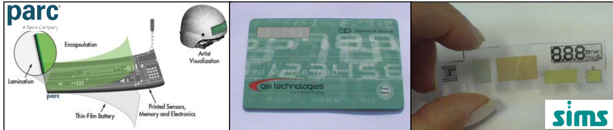
Figure 6 – Integrated Printed Systems under development by several partnerships. PARC blast dosimeter project funded by DARPA (Credit: PARC). One time use pass card (Credit: GSI Technologies). Integrated cholesterol sensor funded by European Union (Credit: SIMS project web page).
