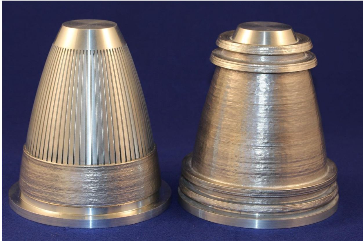
Figure 10. Freeform deposition closeout of nozzle liners, without filler materials.
