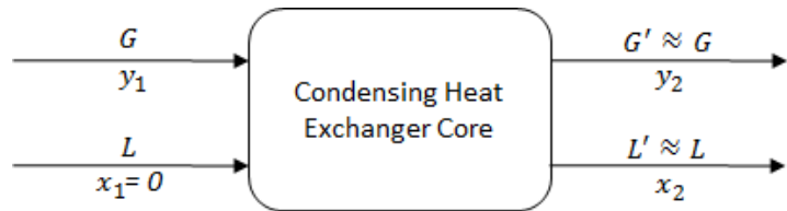
Figure 3. A simplified schematic depicting the condensing heat exchanger mass balance.
