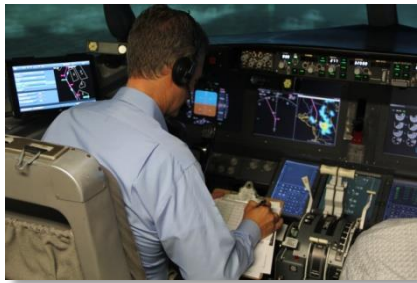
Figure 1. OPL's fixed-base flight deck simulator with the TAP software application to the pilot's left during HITL-2. Photo by M. Cover.
