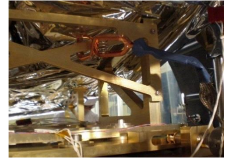
Proposed location of additional harness bracket (at the time, would have been conductive leak from most sensitive heater circuit with least margin)
