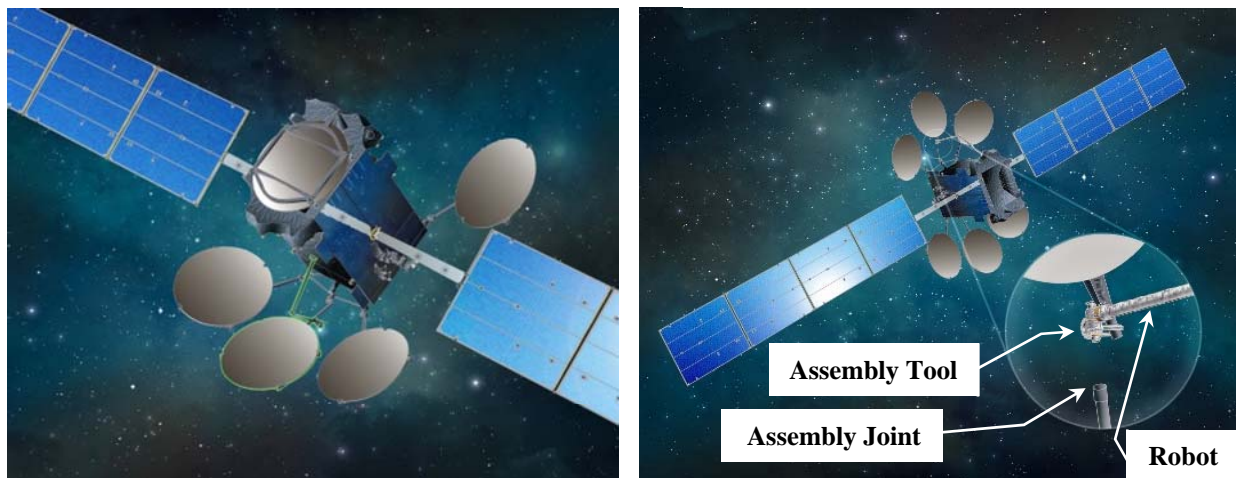
c) First robotically installed reflector secured to operational location.
