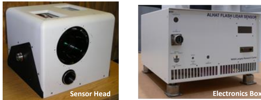
Figure 2. ALHAT Flash Lidar Sensor.
