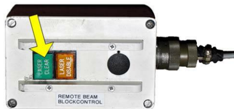
Figure 10: Remote Beam Block Control Box
