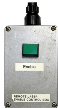
Figure 16: The ENABLE button on the Remote Laser Enable Control box
