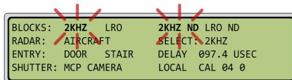
Figure 5: IOC Display showing flashing text indicating that the inserts are in place
