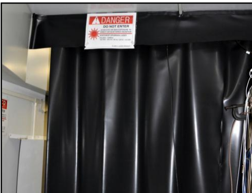
Figure 3-7: Beam blocking curtain inside the shelter
