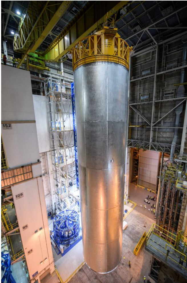
Figure 2. Production of the structural test article of the liquid hydrogen tank for the SLS Core Stage.
