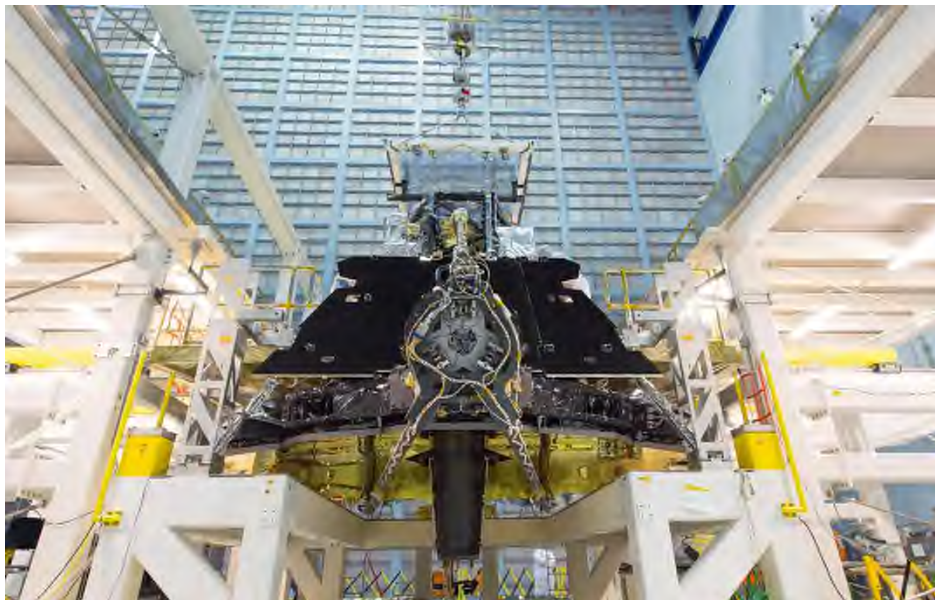
Figure 10. Fully integrated OTIS (OTE + ISIM) in the NASA GSFC Class 10,000 cleanroom
