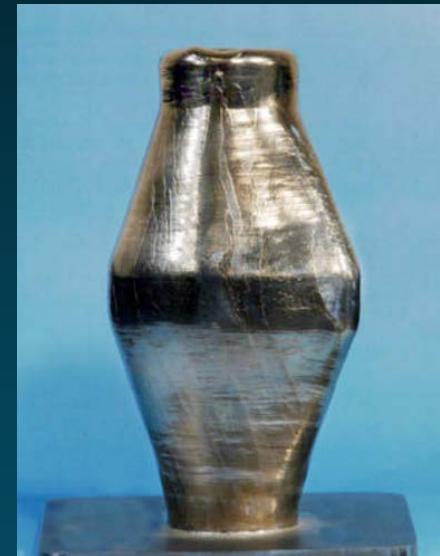
Structural part produced with EBF3 Image credit: NASA
