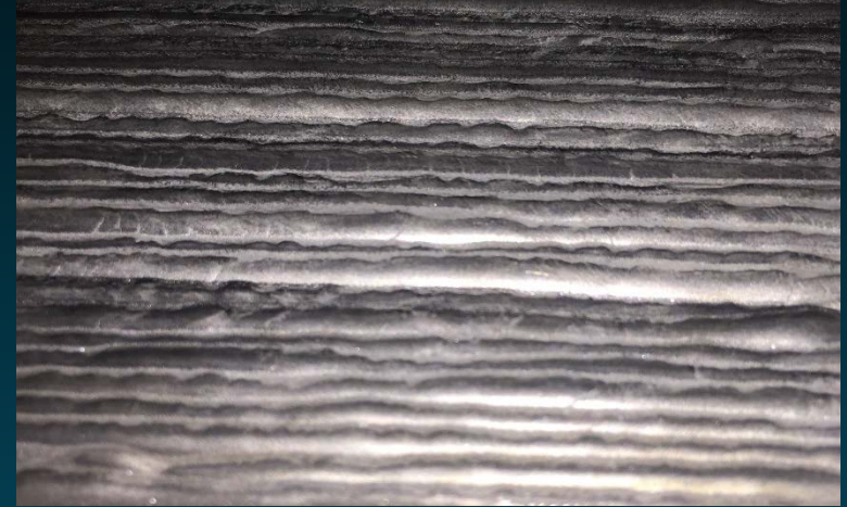
Direct Metal Laser Sintered AlSi10Mg
