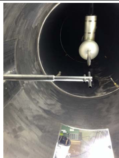
Figure 18: Photo showing ICC mast inserted into the tunnel in front of the IKP2-1 (test 7, Table 2). In this case, a 20 cm cylinder is in front of the IKP2 inlet, and a 10 cm cylinder is beside. All IKP2-1/ICC comparisons use 20 cm pairs. Also shown at bottom is transparent window and video camera used to visualize experiments with polycarbonate cylinders.
