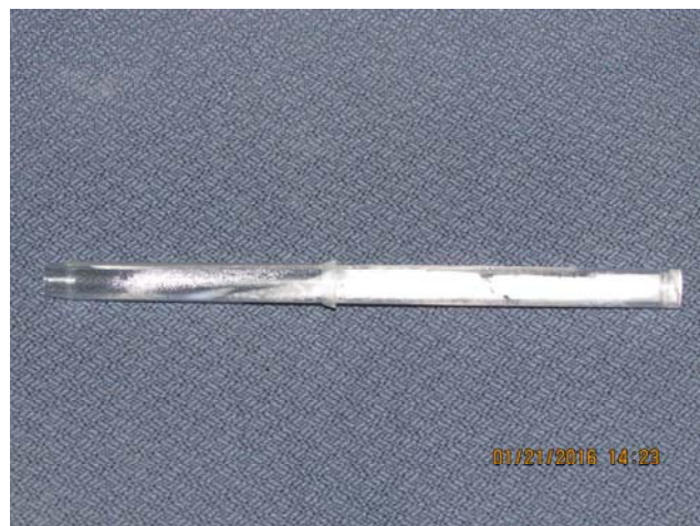
Figure 17: Ice bulk capture using 20 cm transparent polycarbonate cylinder at 150 ms -1 , (test 7, Table 2). The accumulated from the back of the cylinder (right), but the plug was visible at the end of the capture as 2 pieces. Note the thin accumulation of ice at the left on the forward wall near the cylinder
