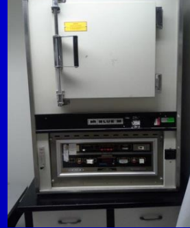
Blue M furnace for high temp synthesis
