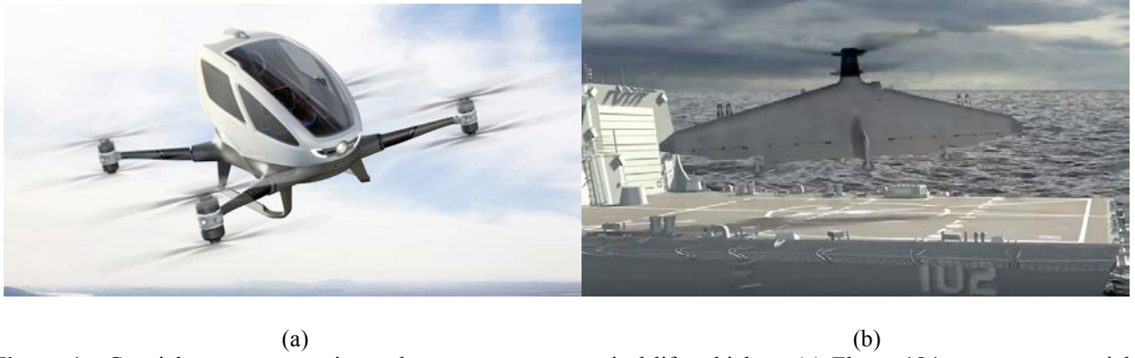
Figure 1. Coaxial rotor systems in modern autonomous vertical-lift vehicles. (a) Ehang 184 autonomous aerial vehicle for human transportation ( www.ehang.com/ehang184 ), (b) DARPA Tern unmanned aircraft system for launch from littoral combat ships ( www.darpa.mil/program/tern ).
