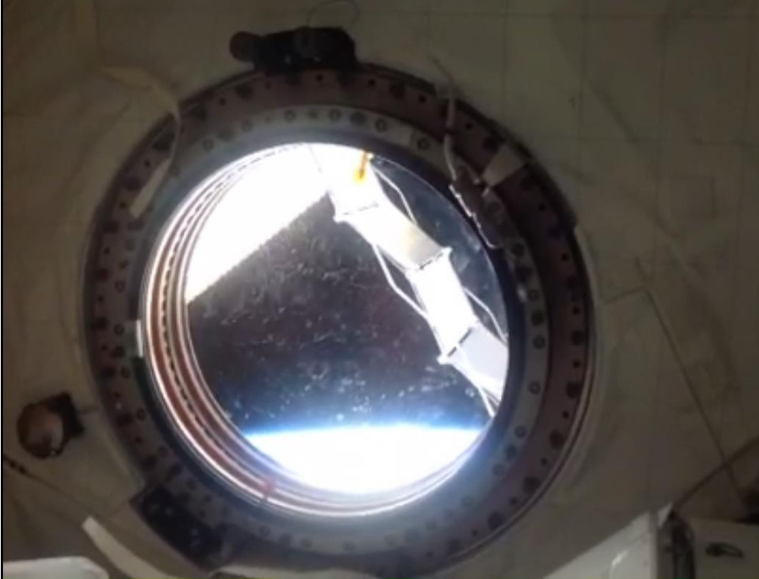
A screenshot from a video showing a scratch pane on an ISS window.
