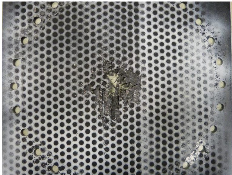
Figure 10. Damage on an un-aged T700/PR520 panel impacted at 531 ft/sec. The damage is localized around the impact point
