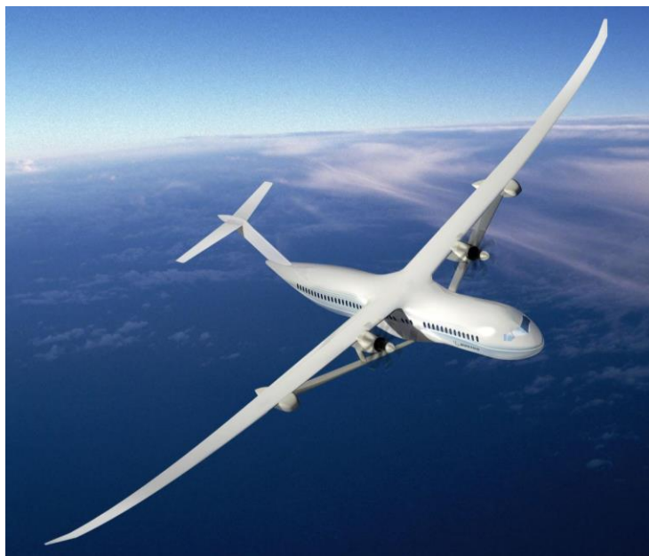
Figure 1. Boeing's SUGAR Volt, hybrid electric-gas propulsion concept.
