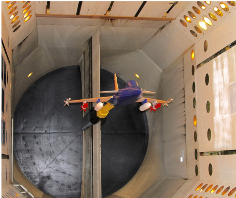
Figure 2. The generic fighter aeroelastic wind-tunnel model installed in the TDT.
