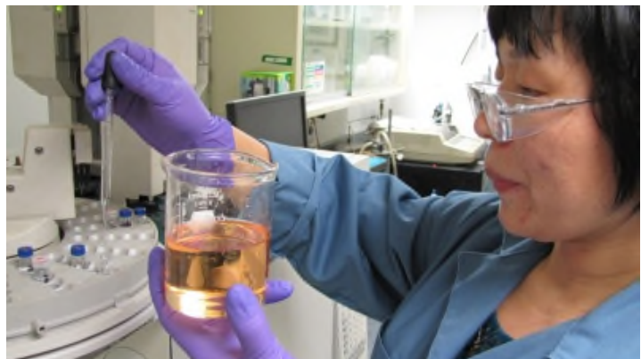
Figure 1. AF-M315E propellant can be safely handled in open containers without need of respiratory protective equipment.
