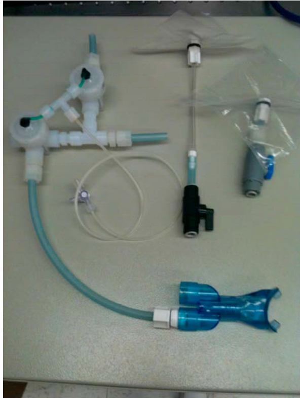
Figure A.9. Prototype MRI-compatible passive gas mixing and delivery device for ventilation imaging in human subjects under voluntary breathing.
