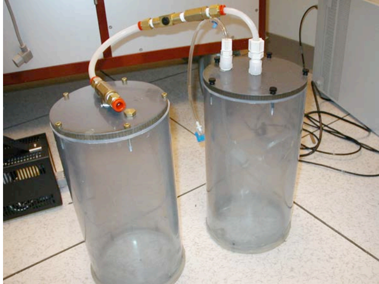
Figure A.5. Hyperpolarized gas chambers scaled up by a two orders of magnitude to accommodate the ventilatory volumes necessary for imaging pigs.
