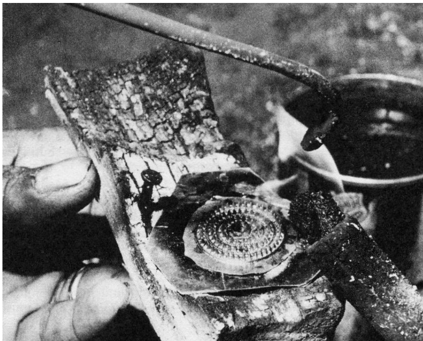
Figure 5.77 Modern use of a mouth blowpipe as a torch (Untracht, Jewelry Concepts and Technology , 349, Fig. 9.36)
