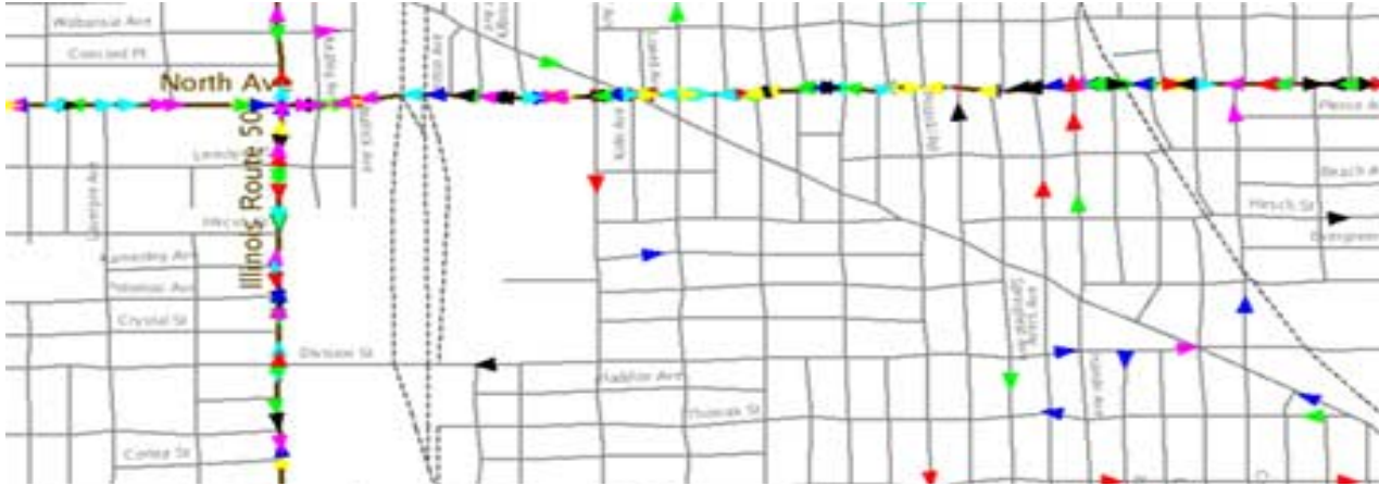
Figure 5. Vehicles routed with least cost paths gradually migrate to higher speed roads in Chicago, IL suburb
