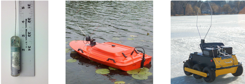
Figure 1.1: Our robotic system consists of radio tags, a radio antenna and receiver mounted on autonomous boat in summer and wheeled rover in winter (to operate on frozen lakes).
