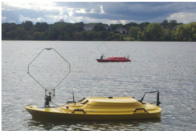
Figure 2.1: The robotic systems used in field experiments. The 2-meter boats were designed to track invasive fish autonomously. Each is equipped with wireless communications, directional antenna used as bearing sensors, a navigation suite, and computing hardware. Our algorithm was implemented on this system and was shown to localize targets to within small uncertainty.
