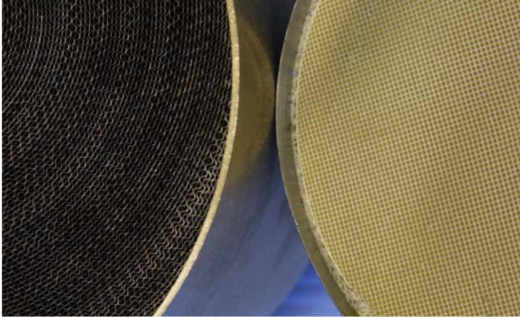
Figure 1.3. Examples of metal-based catalyst (left) and ceramic-based cordierite catalyst (right) (Twigg, 2006).
