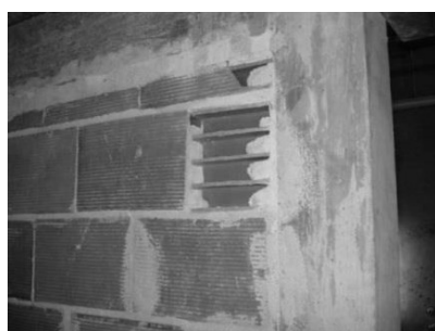
Figure 7.8 Crushing of loaded corner in the test specimen
