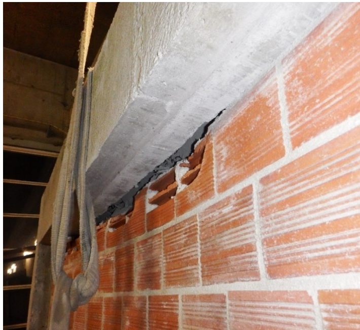
Figure 5.44 Final deformation of the infill; a)total deformation, b)detachment of the wall from bottom rc beam c)detachment of the wall from upper rc beam
