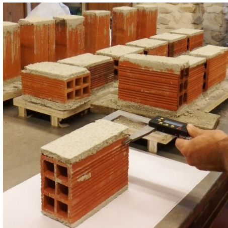
Figure 6.5 Measurement of the dimensions of the bricks
