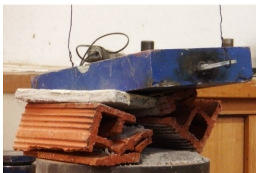
Figure 6.8 Compressive testing of the brick parallel to height a) before test b) after test
