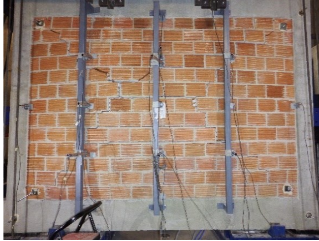
Figure 4.46 Final cracking pattern of the specimen
