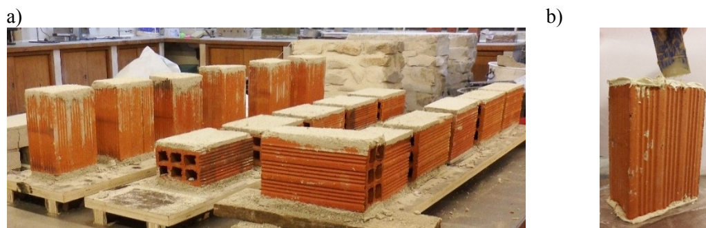
Figure 6.6 Surface preparation of the brick specimens with a) mortar b) polyester
