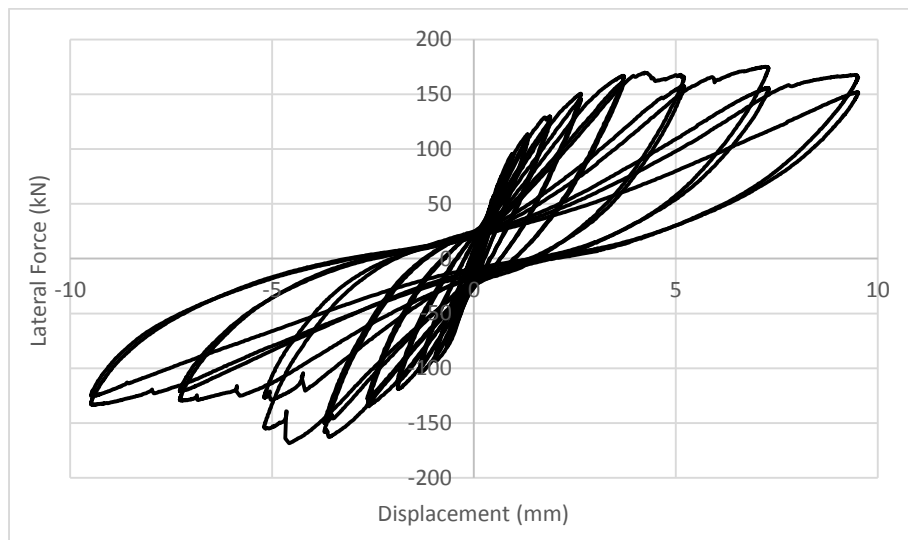
Figure 3.45 In-Plane force-displacement diagram of the specimen SIF-IO(0.5%)-2L(NC)-B
