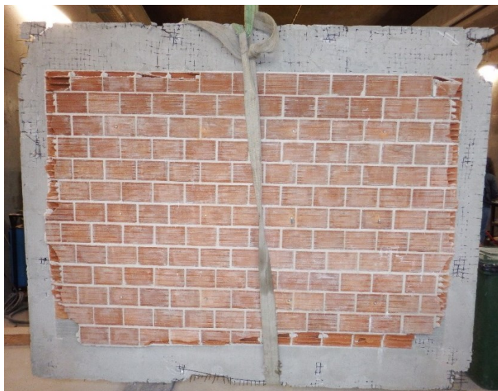
Figure 5.26 External leaf of the brick infill wall crane after the test
