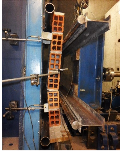
Figure 6.18 Horizontal cracking of the mortar joints due to flexural testing parallel to the bed joints
