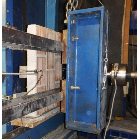
Figure 6.20 Flexural testing of the specimen perpendicular to the bed joints
