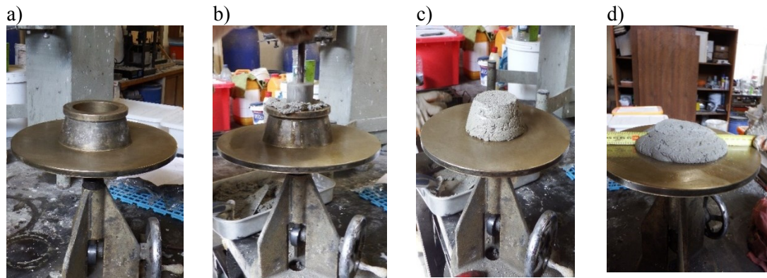
Figure 6.1 Test procedure for evaluation of mortar consistency; a)preparation of the mold b)placing the mortar in the mold and compacting c)removing the mold and jolting the flow table d)measure two vertical diameters of the mortar
