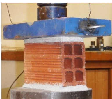
Figure 6.8 Compressive testing of the brick parallel to height a) before test b) after test
