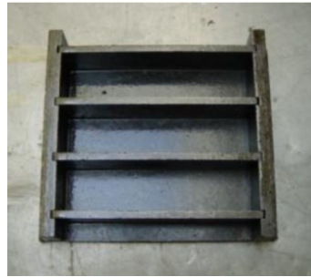
Figure 6.2 Mold used for determining the flexural and compressive strength of mortar
