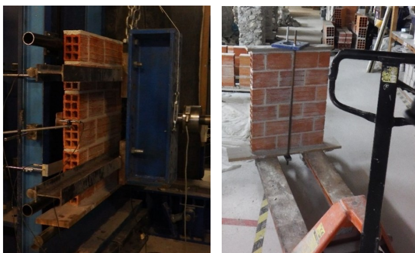
Figure 6.17 Details of experimental testing a) test setup for flexural testing b) transportation of the specimens
