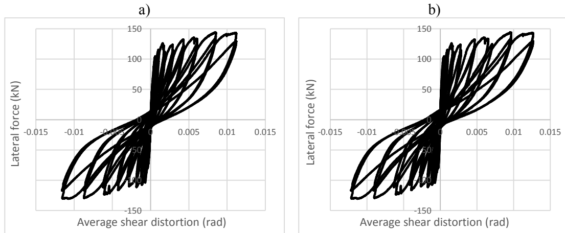
Figure 3.62 Average shear distortion of a) external leaf (8cm thickness) and b) internal leaf (6 cm thickness)
