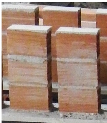
Figure 6.23 Specimens for initial shear test
