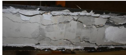
f) Crack pattern in the bottom surface at failure load of SP-3L45 beam
