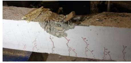
b) Crack pattern at failure load of the R-7S-R beam
