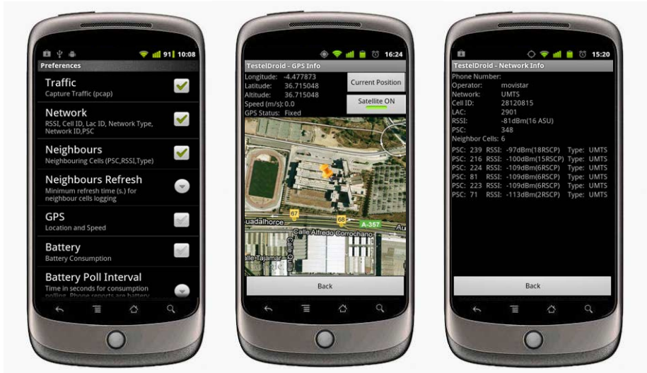
Figure 3.1: TestelDroid screenshots, from left to right: Preferences configuration, GPS measurement localization and Network information
