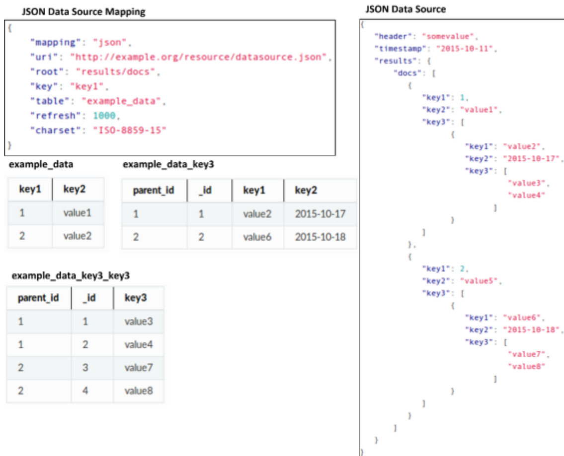
Figure 5. JSON data source example mapping and resulting relational tables
