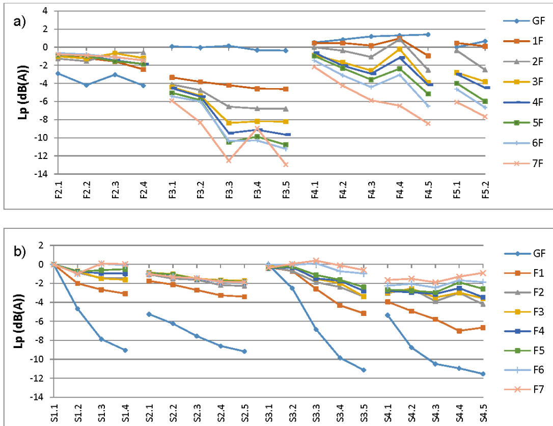
Figure 15: Average exposure at windows. (a) In façade geometry cases. (b) In Street geometry cases.
