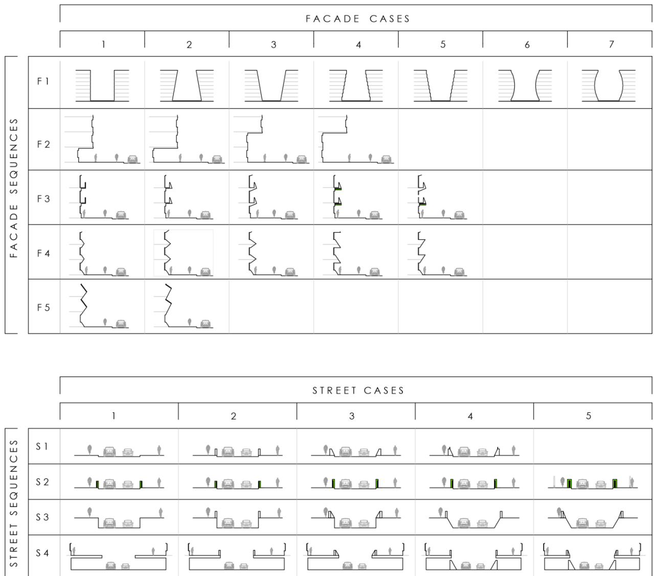
Figure 2: Elements analysed in sequences and cases considered in this study. a) Façade sequences: F1-General building shape. F2-Setback of the lower storeys. F3-Balcony geometry. F4-Triangular prominences on façade. F5-Shielded inclined windows. (b) Street sequences: S1-Low barrier shape. S2-Green absorption on a vertical low barrier. S3-Depressed road. S4-Two level street.
