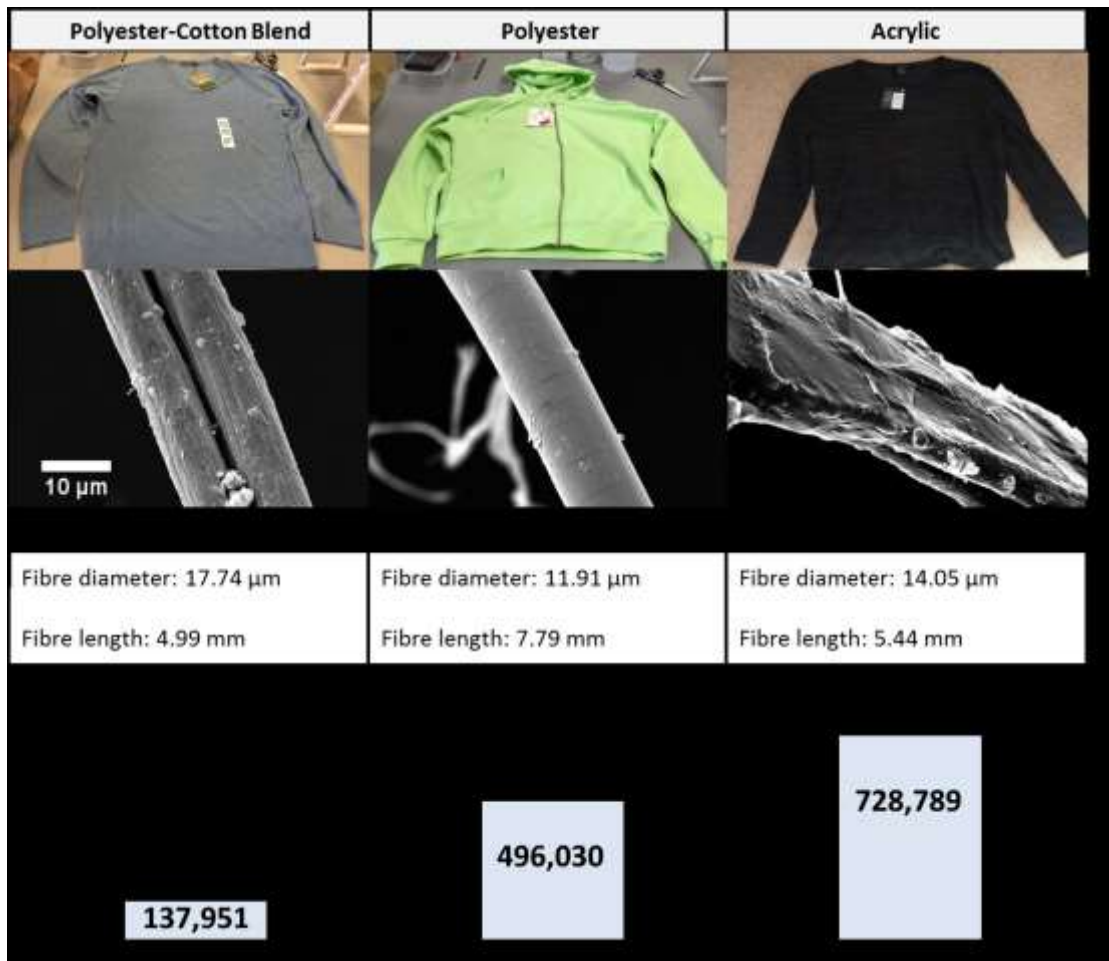
441 Figure 2. Images to show the original garments (each representing a different 442 fabric), and a scanning electron microscopy image (SEM) of a typical fibre 443 from each fabric (the scale bar is consistent for all images - 2500 X 444 magnification). Key details are included below about the mean dimensions of 445 fibres released during laundering, and estimated quantity released from the 446 fabric during each wash (assuming a typical washing load of 6kg).
