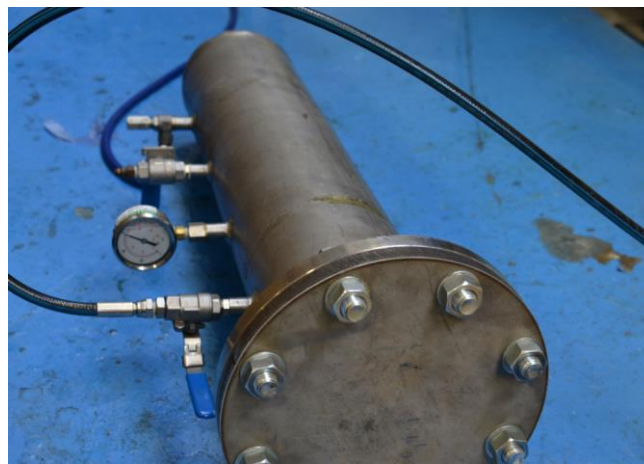
Fig.3. The hydrostatic chamber used in the diffusion test.
