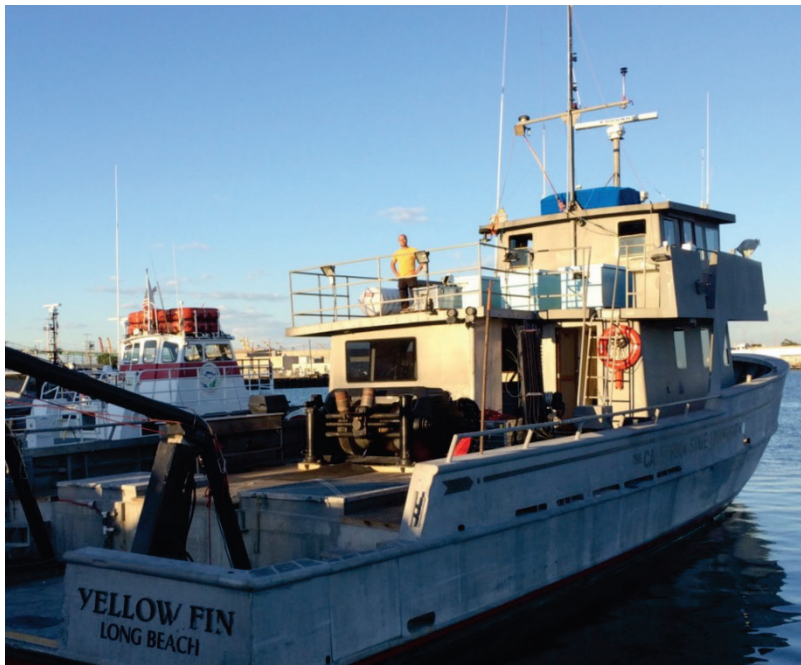
Figure 1. The research vessel Yellow Fin that was used for tracking ships from open sea to berth at the harbor to investigate emissions at various modes of operation. The sample inlet and the wind meter are mounted on the opposite ends of the mast's horizontal yard.
