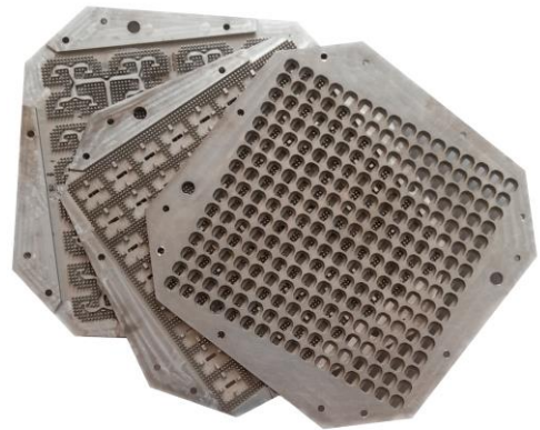
Fig. 4. Photograph of the proposed 16 \times 16 slot array antenna fabricated by die-sink EDM.
