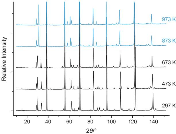
**Figure 3:** Stacking plot of temperature-dependent diffractograms of  $\text{Li}_{0.7}\text{TiS}_2$  (normalized to the intensity of the niobium (011) reflection at ca.  $38.5^\circ$ ). 1T phase in black, 3R phase in blue/grey, container reflections cut off at high intensities for clarity.
