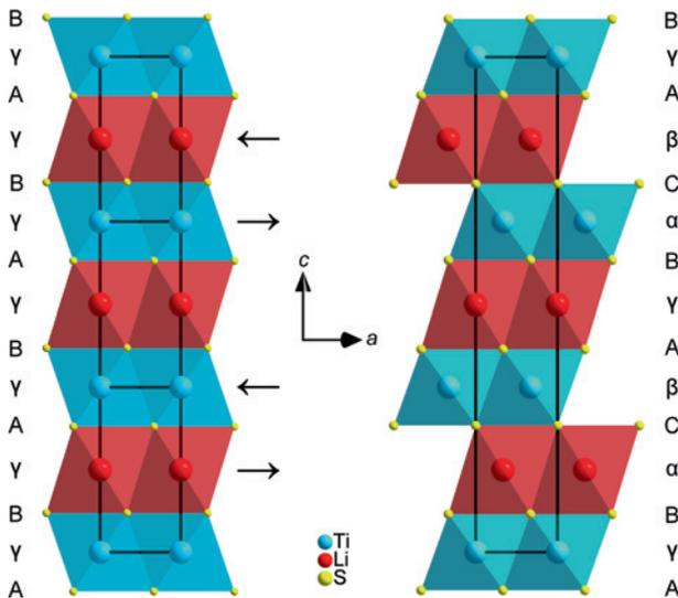
**Figure 1:** Crystal structures of 1T- (left) and 3R- $\text{LiTiS}_2$  (right). View along  $[010]$ , unit-cell edges in black, stacking sequences at the margins, arrows indicating the hypothetical movement during the transformation  $1\text{T} \rightarrow 3\text{R}$ .
