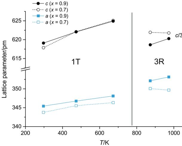
**Figure 4:** Temperature evolution of the lattice parameters.  $a$  in blue/grey as squares,  $c$  in black as circles (value divided by three in the 3R regime).  $\text{Li}_{0.7}\text{TiS}_2$  with hollow symbols and dashed lines,  $\text{Li}_{0.9}\text{TiS}_2$  with solid symbols and lines. Lines merely guiding the eye.
