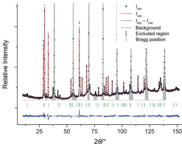
**Figure 2:** Exemplary neutron diffractogram of 1T- $\text{Li}_{0.9}\text{TiS}_2$  at 673 K with fit and background data.
