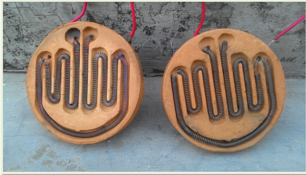
Fig 3.2: Re-designed coil for 2 stoves
