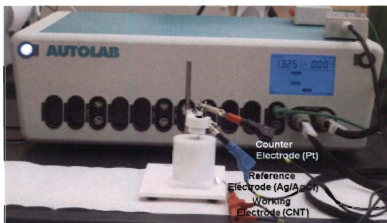
Figure 6.2 Photograph of the three electrode instrumental set-up used for electrodeposition.
