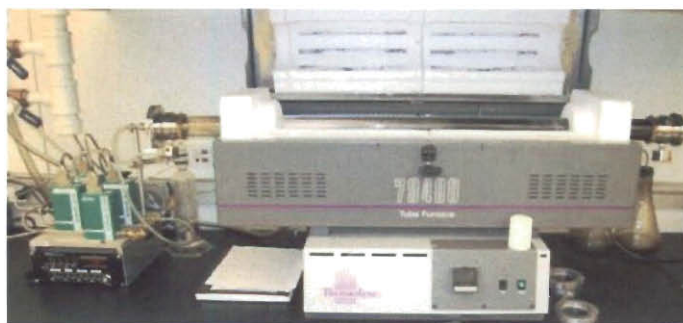
Figure A.7 Photograph of the CVD system used for CNT growth
