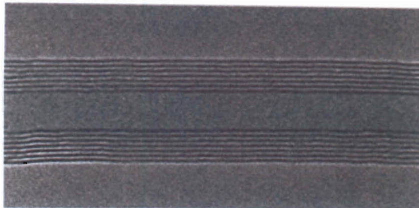
Figure 2.7 HRTEM image of a MWCNT showing the multiple layers. The interlayer distance is 0.34nm. (Ajayan et al. Reports on Progress in Physics, 1997, 60)
