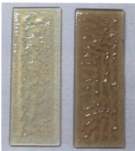
Figure 5.9 Photograph of Fe-PDMS film before and after the heat treatment. The color change indicates the formation of iron nanoparticles.
