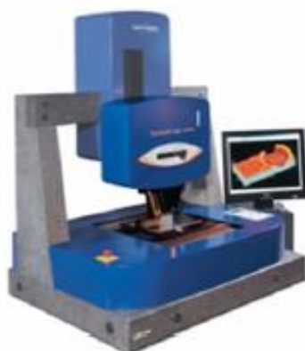
Figura 5.1: profilometro TalySurf CLI 2000 Taylor Hobson
