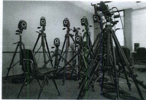
Figure 3.2 : Vicon motion capture system used in the experiments to capture the trajectories of the markers depicted in Fig. 3.1.
