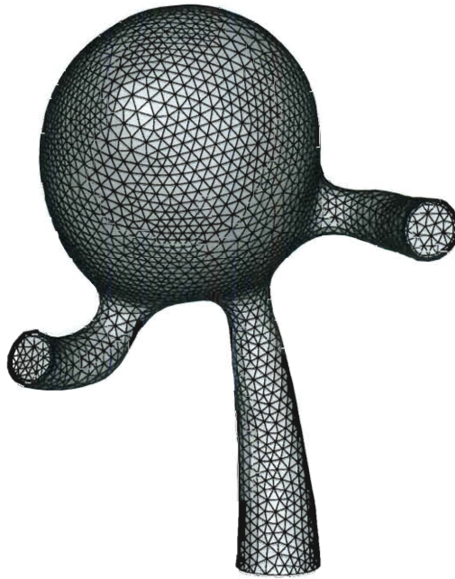
Figure 5.4: Fluid mechanics mesh of tetrahedral elements at starting pressure.
