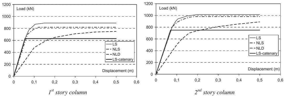
Fig. 9. Progressive collapse resistance of the 2-story structure ( $COV_m = 7\%$  and  $COV_l = 10\%$ ) designed according to M.D. 08.
