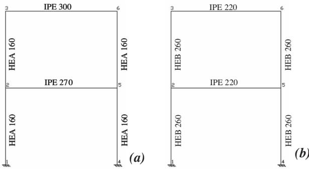
Fig. 5. 2-Story frame designed according to M.D. 96 (a) and M.D. 08 (b) Italian codes.
