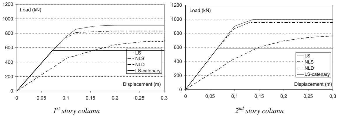
Fig. 8. Progressive collapse resistance of the 2-story structure ( $COV_m = 7\%$  and  $COV_l = 10\%$ ) designed according to M.D. 96.
