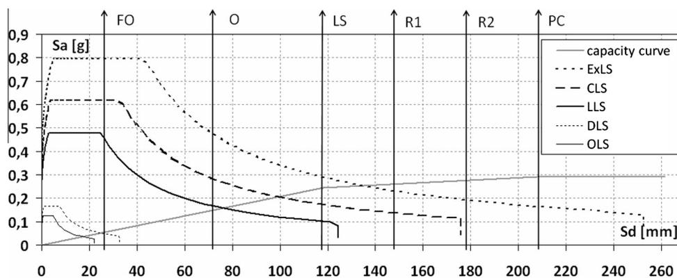
Fig. 7. Characteristic pushover curve of the 2-story frame designed according to M.D. 08.
