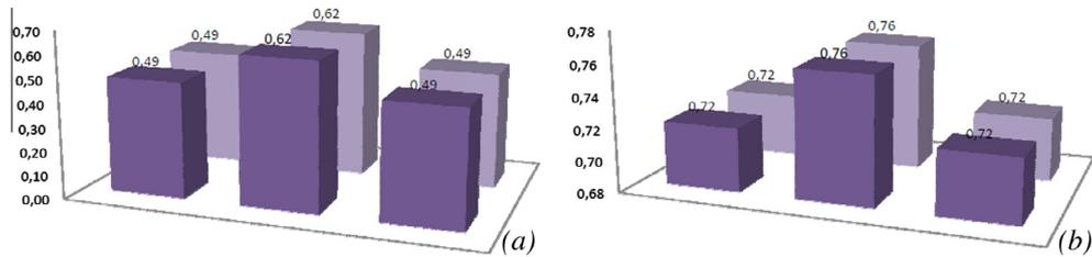
Fig. 15. Robustness indices of the DM 96 structure type A with rigid and full strength connections at the first level (a) and the second one (b).
