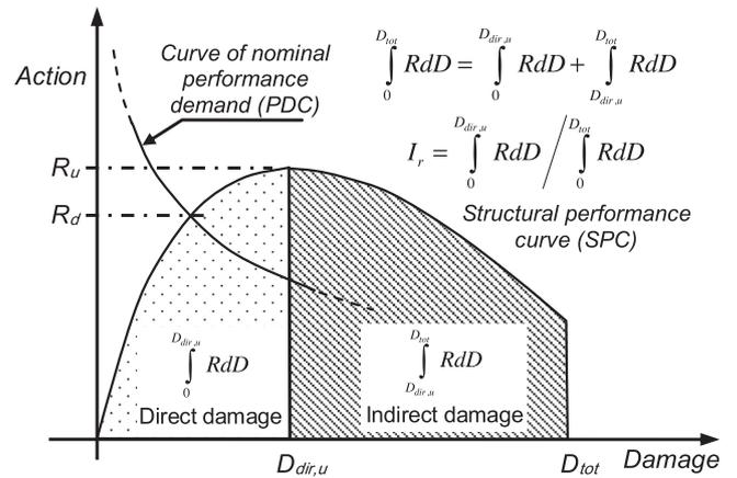
Fig. 3. Definition of direct and indirect damaged.
