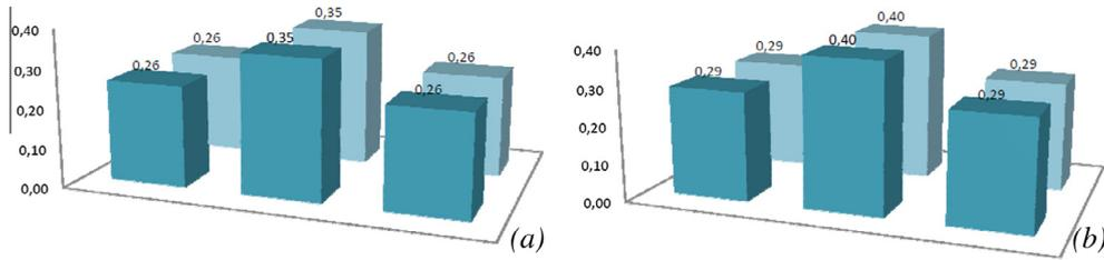
Fig. 17. Robustness indices of the DM 96 structure type A with semi-rigid and partial strength connections at the first level (a) and the second one (b).
