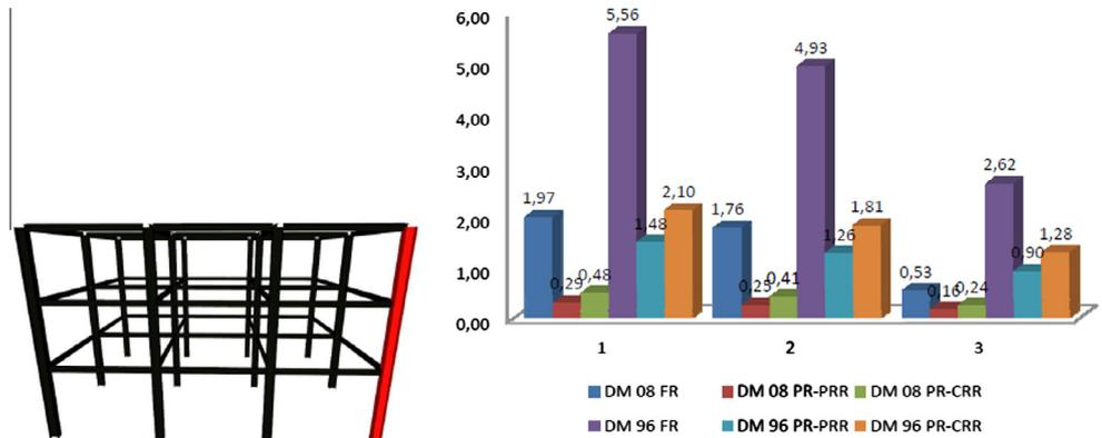
Fig. 20. Robustness indices of the structure type B with removal of a corner column.
