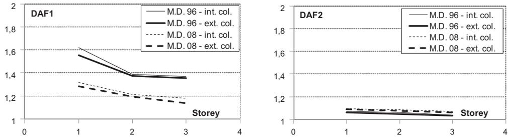
Fig. 12. Change of DAFs with respect to the column removal at different stories.
