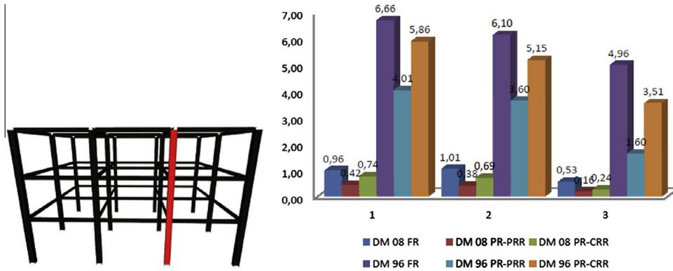
Fig. 21. Robustness indices of the structure type B with removal of one perimeter column on its long side.
