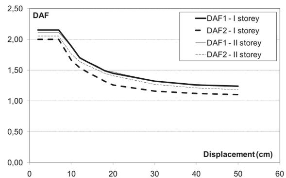
Fig. 11. DAF vs. displacement demand for the 2-story structure designed according to M.D. 08.
