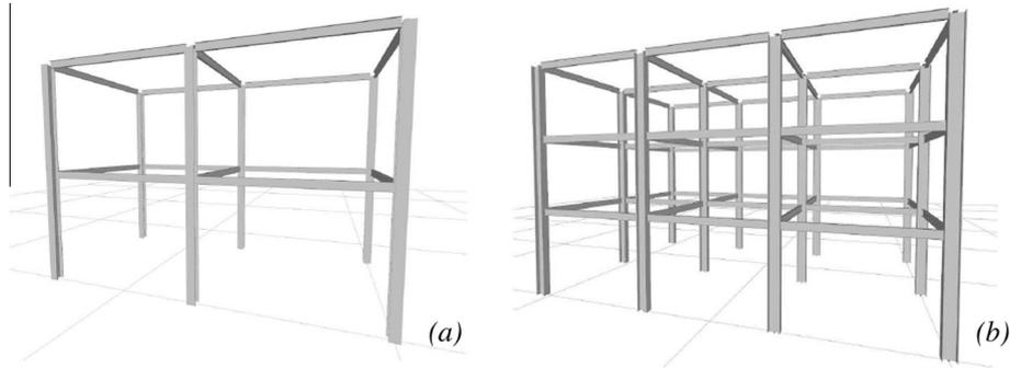
Fig. 13. 3D FEM models of type A (a) and type B (b) structures.
