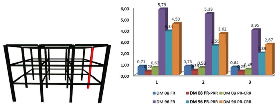
Fig. 22. Robustness indices of the structure type B with removal of one perimeter column on its short side.
