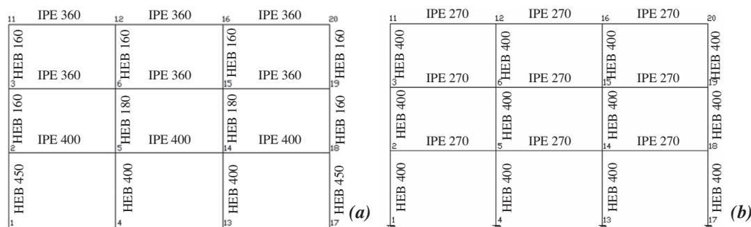
Fig. 6. 3-Story frame designed according to M.D. 96 (a) and M.D. 08 (b) Italian codes.
