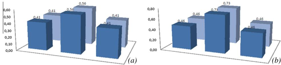
Fig. 14. Robustness indices of the NTC 08 structure type A with rigid and full strength connections at the first level (a) and the second one (b).
