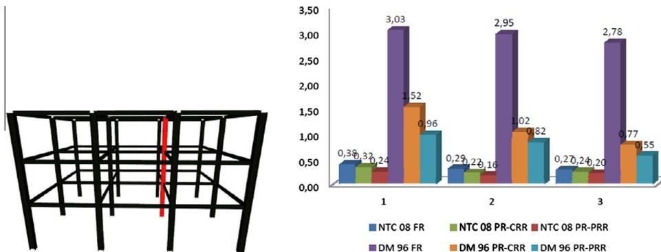
Fig. 23. Robustness indices of the structure type B with removal of a central column.
