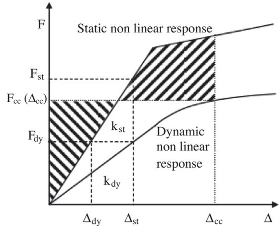
Fig. 4. Static non linear response curve vs. dynamic non linear one and explanation of the DAF.
