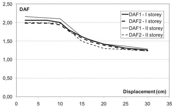
Fig. 10. DAF vs. displacement demand for the 2-story structure designed according to M.D. 96.
