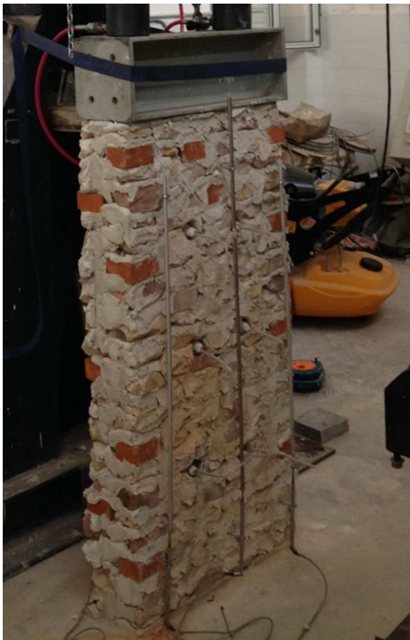
Fig. 8 Compression tests on reinforced panel 4Rf
