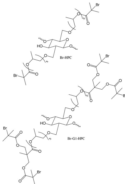
**Figure 11:** Molecular structure of macro-initiators Br-HPC and Br-G1-HPC
