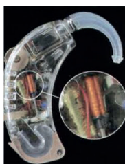
Figure 1 'Telecoil' in hearing aid
