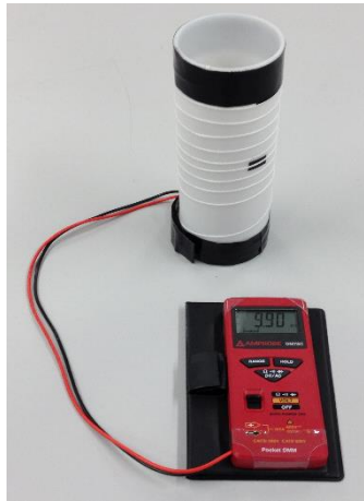
FIGURE 7. 31: A PROTOTYPE THERMISTOR E - YARN
