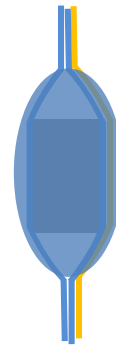
FIGURE 6. 156: SCHEMATIC OF THE SIDE VIEW OF THE MICRO POD WHEN THE CARRIER YARNS ARE EITHER SIDE
