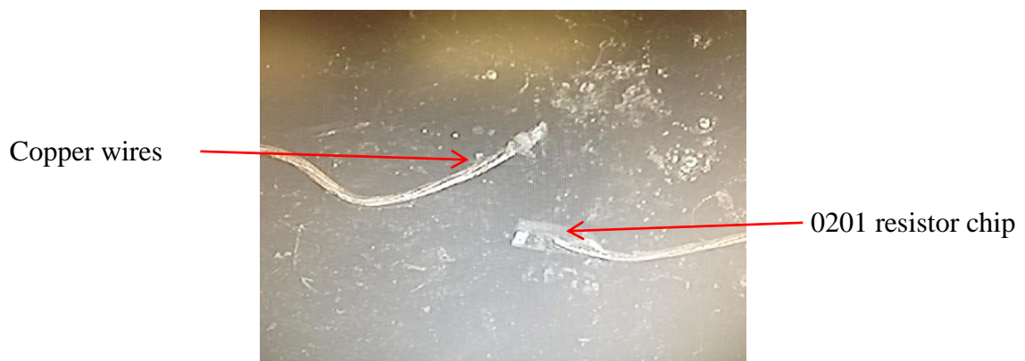
FIGURE 4. 19: SOLDER JOINT FAILURE AFTER SOLDERING OF 0201 RESISTOR WITH 7 STRAND COPPER WIRE
