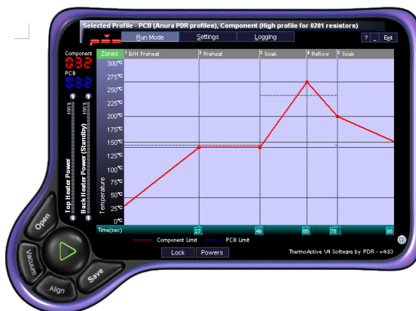
FIGURE 4.17 C: HEATING PROFILE
