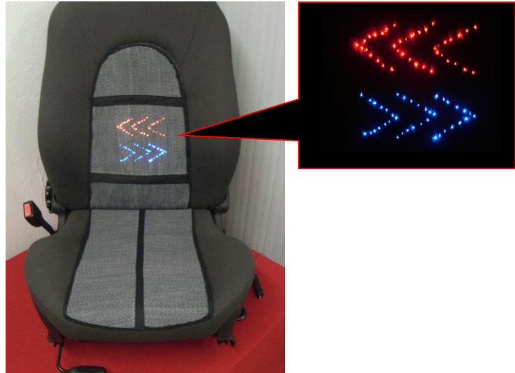
FIGURE 7. 10: THE PROTOTYPE DEMONSTRATOR OF AN ILLUMINATED CAR-SEAT COVER
