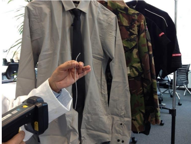
FIGURE 7. 50: RFID E-YARN AND RFID E-YARN-INTEGRATED GARMENTS 7.6.5 Washing of RFID e-Yarn Integrated Garment
