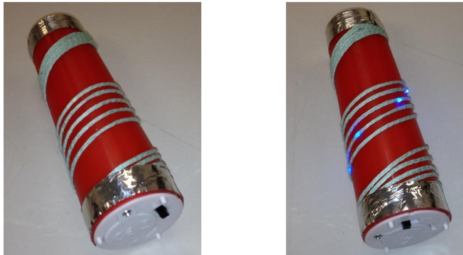
FIGURE 7. 2: E-YARNS CONTAINING BLUE LED'S BEFORE AND AFTER ACTIVATION
