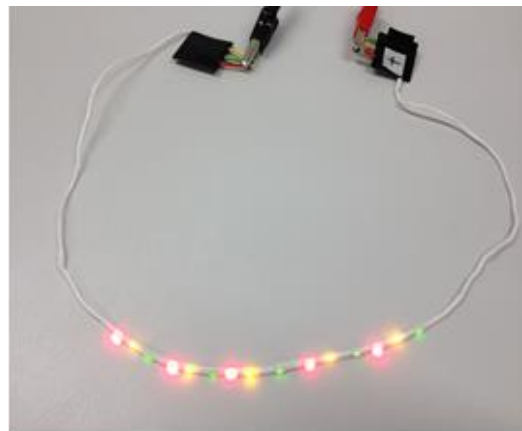
FIGURE 7. 9: THREE- COLOUR ILLUMINATED YARN
