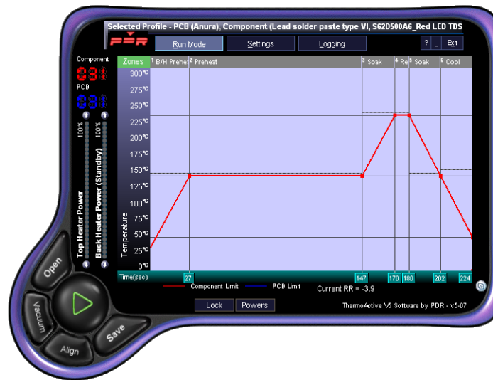
FIGURE 4. 3: THE USER INTERFACE OF THE CONTROL SOFTWARE OF THE PDR IR REWORK SYSTEM
