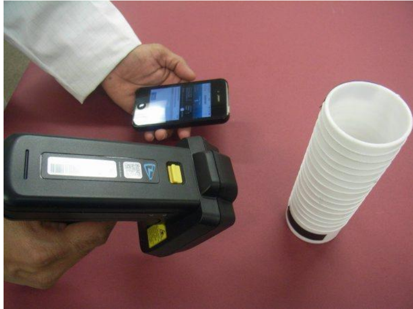
FIGURE 7. 49: TESTING OF RFID E-YARN USING AN RFID READER AND IPHONE APP
