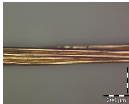
FIGURE 3. 5: UNCOATED 8 STRANDS COPPER WIRE
