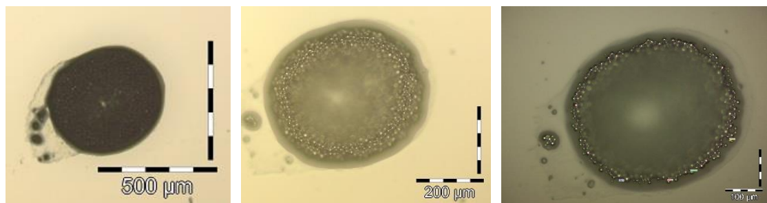
FIGURE 3. 22: MICROSCOPE IMAGES OF SN96.5AG3.0CU0.5 TYPE VI SOLDER PASTE
