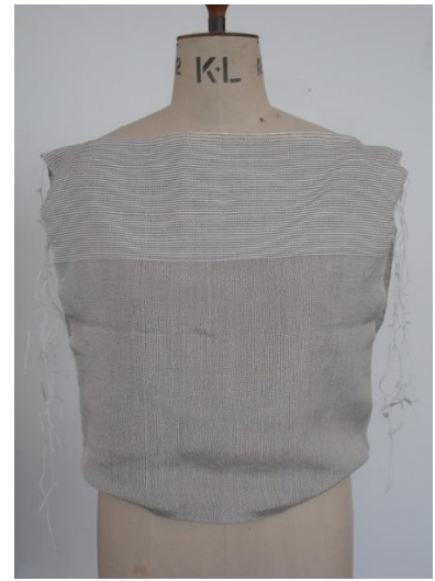
FIGURE 7. 23: THE GARMENT JUST AFTER REMOVAL FROM WEAVING LOOM
