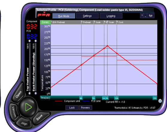
FIGURE 4.17 D: HEATING PROFILE
