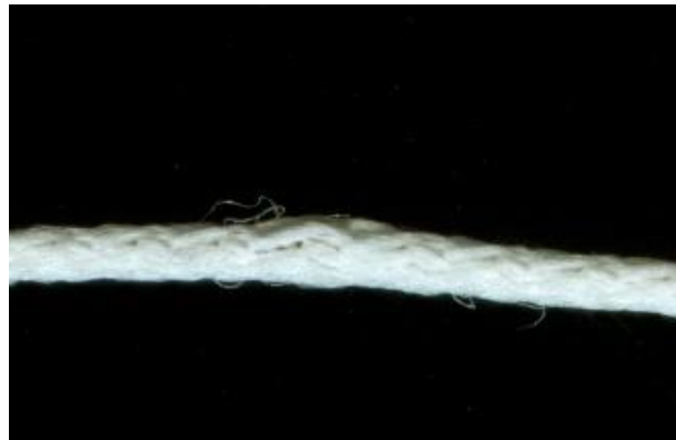
FIGURE 6. 13: A PICTURE OF E-YARN WITH MICRO POD BEING PUSHED UP TO THE YARN SURFACE
