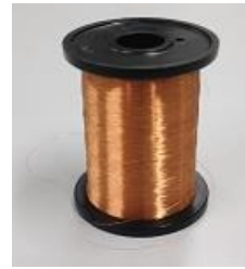
b. Coated single strand copper wire A
