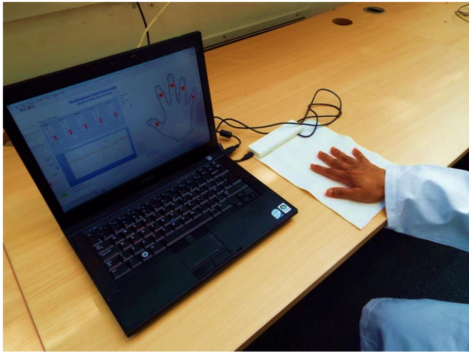
FIGURE 7. 39: DEMONSTRATION OF THE RESPONSE WHEN ALL FIVE FINGERS OF THE AUTHOR’S HAND ARE IN CONTACT WITH THE TEMPERATURE-SENSOR FABRIC MAT
