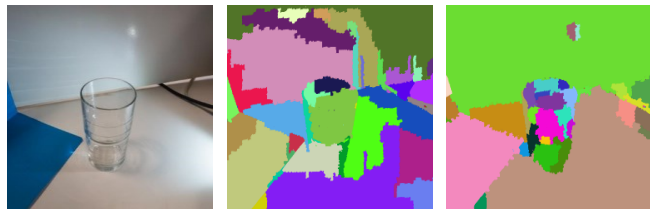
Figure 3: Incorporating edges on the graph segmentation. Left : Original image. Center : standard super-pixel segmentation. Right : our edge-enhanced graph segmentation produces less noise, less spill (note base of glass) and overall better outline of the objects.
