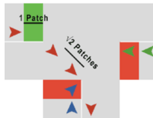
Figure 2. Close-up of intersection, showing distance travelled by a vehicle when moving straight or turning across the intersection
