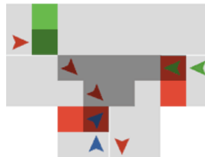
Figure 3. Close-up of intersection. The darker colours show patches in the intersection which are either at a traffic light, or are crossed by more than one traffic flow
