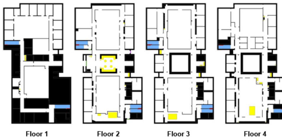
Figure 3. Layout of the Human Services Research Center (HSRC). Exits on Floor 2 are shown in green and red, stairways are shown in blue. North is up in the illustration.
