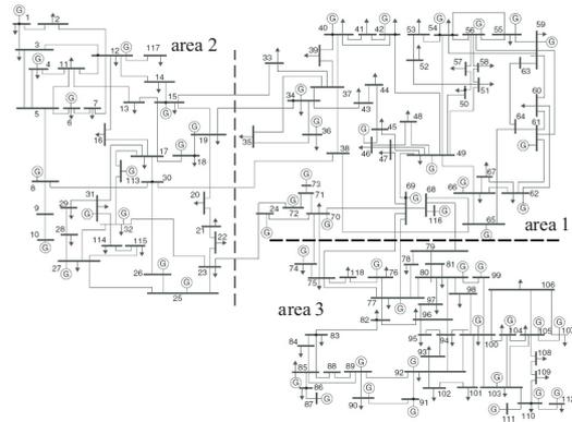
Figure 1: IEEE 118 bus system with 3 TSOs.
